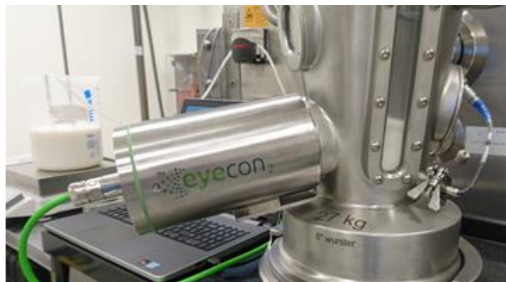
Figure 3 – Eyecon2 in-place on the product container window
